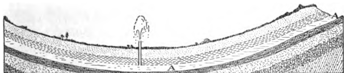
FIG. 105. — Artesian Basin, Showing Arrangement of Rock Strata.
